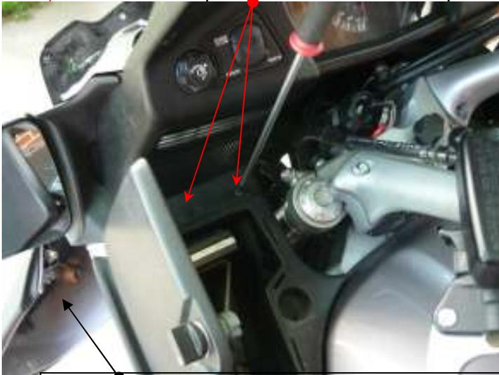
6) Remove 4 Phillips screws from instrument panel 2-L side 2-R side
