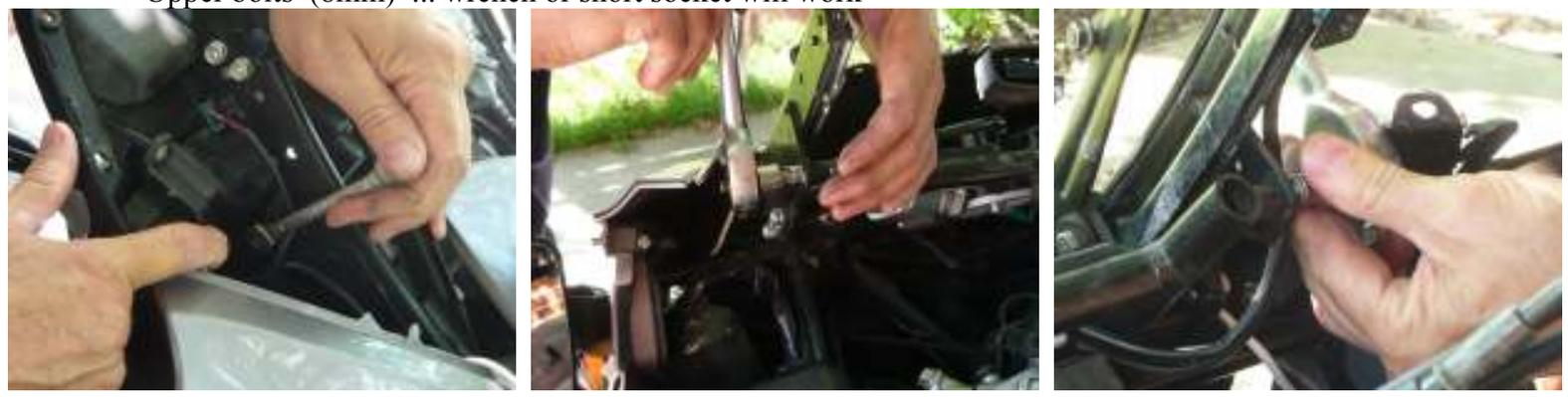
14) Remove the window adjustemnt mechanism electrical connection by first pushing the white plastic clip portion through the frame .....once the connector joint is free from the frame, seperate the connector as shown
