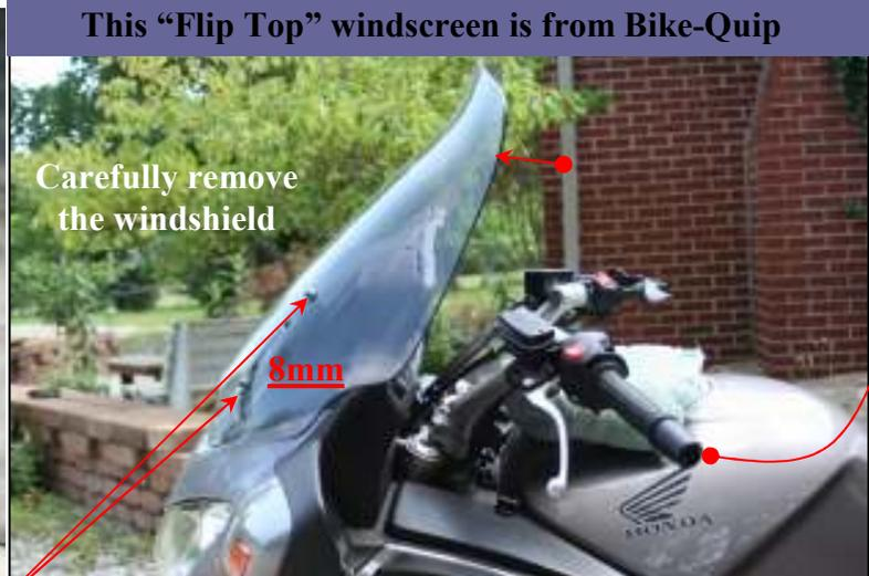
\* Alternately (if stuck in lower positions) 1st remove windshield from brackets 4 (8mm) bolts (2L,2R) then go back to step#3; "remove brackets from window arms".
