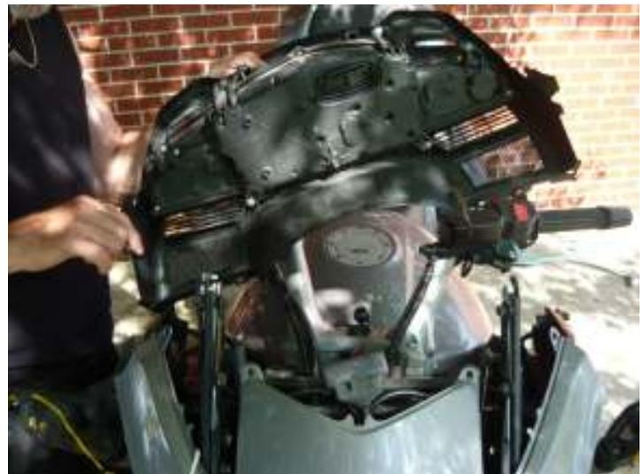
With the Windshield, Dash and Nose piece removed, you can start to see that the hardest part of disassembly is over. Take a breath....maybe have a cold one. A few more bolts will have the window adjuster assembly out and on the bench for cleaning and drive gear replacement.
